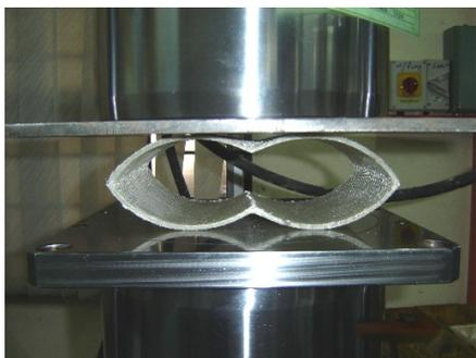
Fig. 3 Formation of fracture longitudinal lines for CCT specimen
