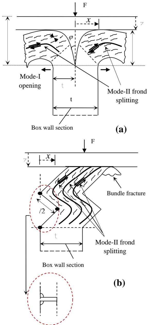
Fig. 1. Ideal crush zone, (a) Lamina bending/brittle fracture crushing mode and (b) Local buckling/transverse shearing crushing mode.
