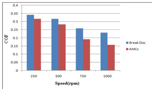
Figure 2-a: Comparison of COF Vs speed Between AMCs and brake disc
