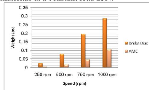
Figure 1-a: Comparison of weight loss between brake disc and AMCs, at 25N
