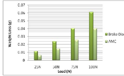
Figure-3 Comparison of weight loss Vs load
