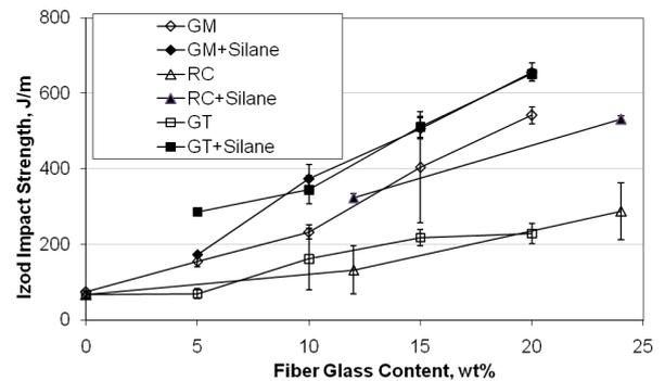
**Figure 1; Izod impact strength for UPVC composites<sup>1</sup>.**
