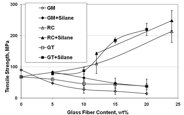
**Figure 2; Tensile strength for UPVC composites<sup>1</sup>.**
