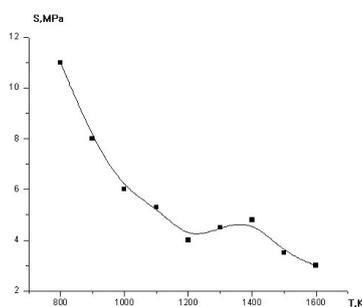
Fig.1 Dependences of the electrical conductivity (a) and proof strength (b) of composites, based on polyformaldehyde and epoxy resins, polymethylsilsesquioxane and glassy fiber, on the pyrolysis temperature
