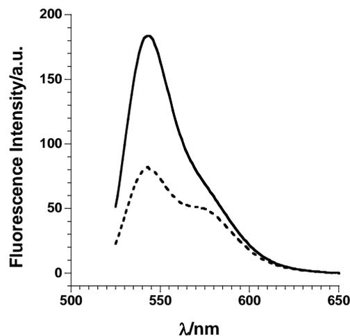
**Fig. 3.** Close and open of the nano-tweezers by UV (solid line) and visible light (dotted line) irradiation at 50 °C.
