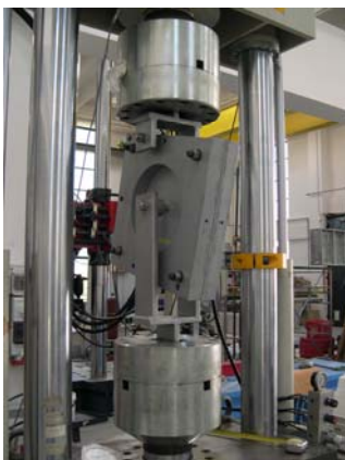
Fig. 3: Fixture attached to Shenck Hydropuls servo-hydraulic testing machine.
