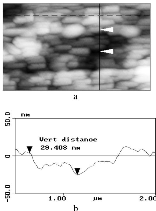
FIGURE 3. a. AFM topography image of the scanned area shown in figure 2. b. Its line profile analysis.
