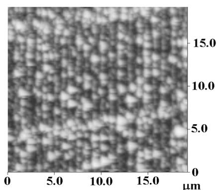
FIGURE 1. AFM image of the  $\langle 110 \rangle$ -axis oriented YBCO film surface.
