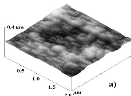
FIGURE 2. AFM 3D image of the  $\langle 110 \rangle$ -axis oriented YBCO film surface.
