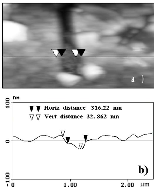
**FIGURE 4.** AFM Image of a scratch carried out on  $\langle 110 \rangle$ -axis oriented YBCO film using a load of  $P=10 \mu\text{N}$ . a) Scratch image. b) Its section analysis.
