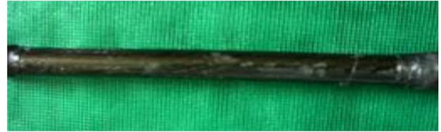
Fig 5: Static test specimen showing failure mode for carbon/epoxy tube with  $[0/90^\circ]$  stacking sequence.
