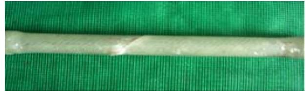
Fig 4: Static test specimen showing failure mode for glass/epoxy tube with  $\pm 45^\circ$  stacking sequence.
