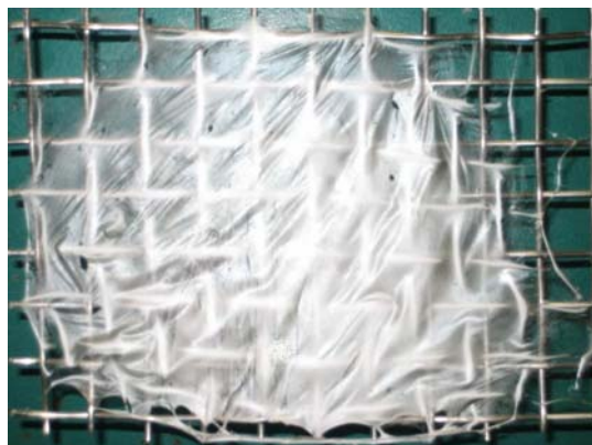
Fig. 3 - Polymer mat on mesh electrode collector
