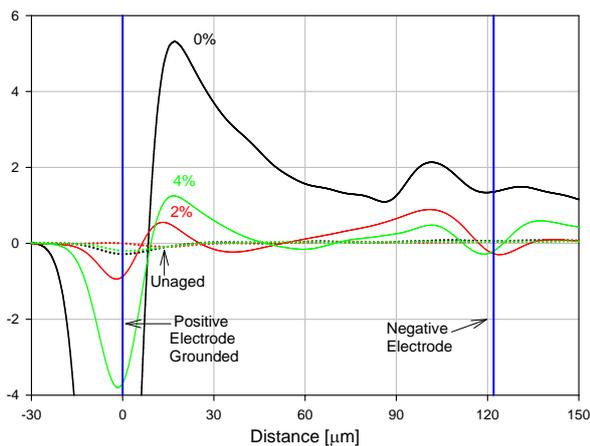
Fig. 2. Space charge distribution in the three materials: unaged (dotted curves) and aged for 120 h (solid curves).
