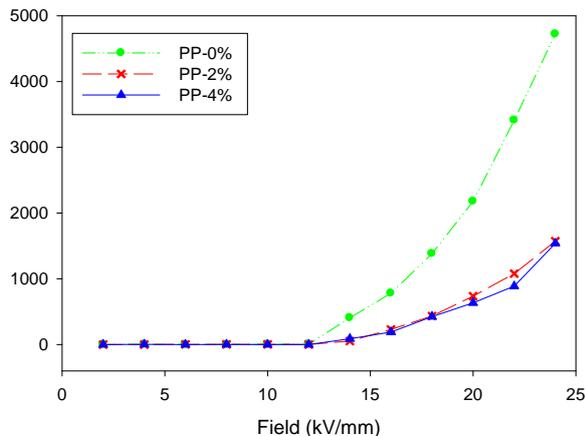
Fig. 1 EL emission in the three materials as a function of the of the ac electric field
