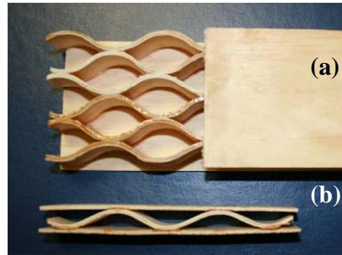
Fig.1 Corrugated cores: (a) single corrugation, (b) multiple-corrugation honeycomb.
