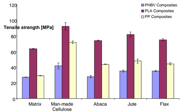
Fig. 2: Comparison of Tensile strength
