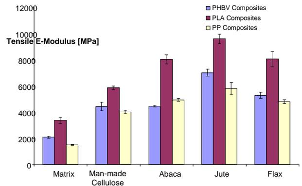
Fig. 1: Comparison of Tensile E-Modulus of different fiber types vs. matrix
