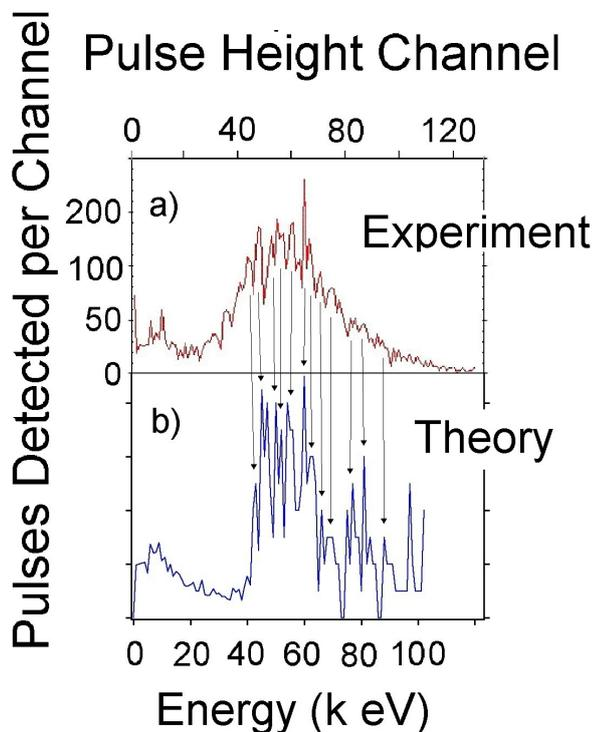
Fig. 1 The pulse height spectra of 15% Gd doped HfO<sub>2</sub> on n-type Si(100) samples with thermalized neutrons from a PuBe source with a flux of 600 neutrons s<sup>-1</sup> incident on the diode, compared to expectations.
