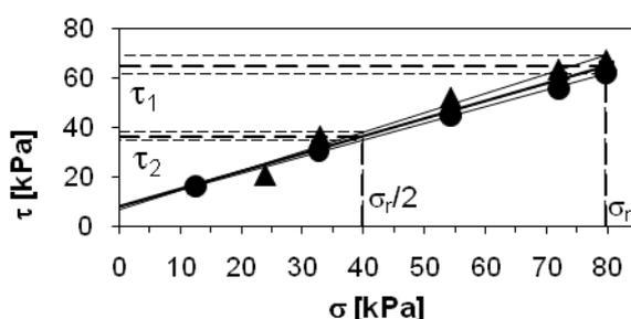
Fig. 1 Relations shear stress – normal stress of tested materials ( -raw, - S\_18, - S\_SH15).
