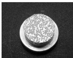
Fig. 2. The measurement of the adhesive force - array composed of particles placed on a tacky surface.
