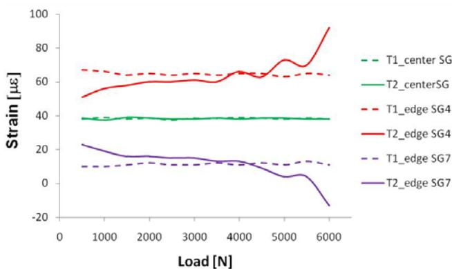
Figure 2 – Strain gages increments versus load for T1 and T2 type of tests
