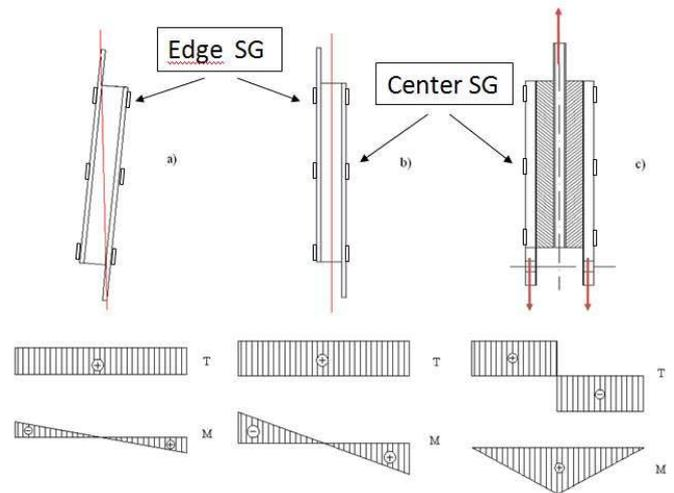
Figure 1 – Load lines and trends of bending moment  $M$  and shear stress  $T$  for the three types of tests: a) T1 b) T2, c) T3.
