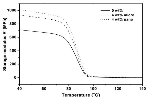
Fig.2 Storage modulus E' versus temperature of PS/Al<sub>2</sub>O<sub>3</sub> composites at 4wt% nano and micro Al<sub>2</sub>O<sub>3</sub>.
