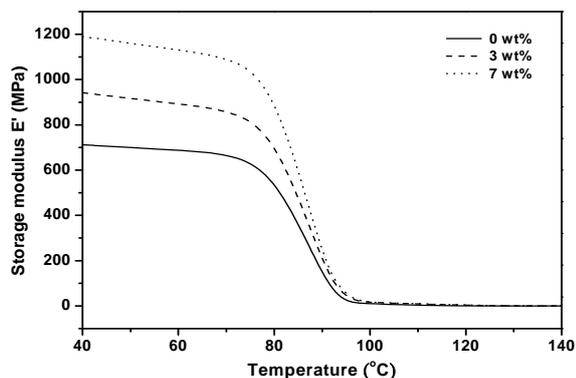
Fig.3 Storage modulus E' versus temperature of PS/nano-Al<sub>2</sub>O<sub>3</sub> composites at various nano Al<sub>2</sub>O<sub>3</sub> contents.
