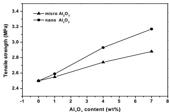
Fig.1 Tensile strength versus nano and micro Al<sub>2</sub>O<sub>3</sub> content of PS/Al<sub>2</sub>O<sub>3</sub> composites.
