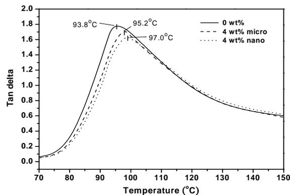
Fig.4 Dynamic tanδ versus temperature of PS/Al<sub>2</sub>O<sub>3</sub> composites at 4wt% nano and micro Al<sub>2</sub>O<sub>3</sub>.
