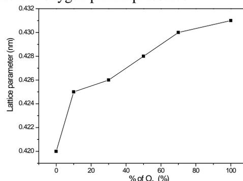
Fig.4 Lattice parameter of NiO films which deposited in different oxygen partial pressures.
