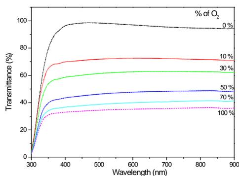
Fig.2 Spectral transmittance of NiO films which deposited in different oxygen partial pressures.
