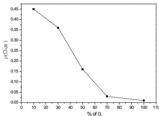
Fig.1 Resistivity of NiO films which deposited in different oxygen partial pressures.
