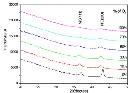
Fig.3 XRD patterns of NiO films which deposited in different oxygen partial pressures.
