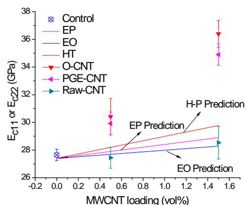
Figure 1. Effect of direct incorporation of MWCNTs into prepreg system by Chen et al. [1]
