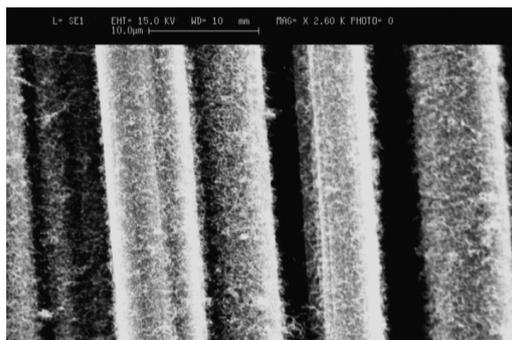
Figure 2 Sparse CNT growth on carbon fiber
