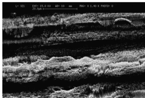
Figure 4 Aligned CNT growth on carbon fiber
