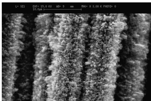
Figure 3 Dense CNT growth on carbon fiber
