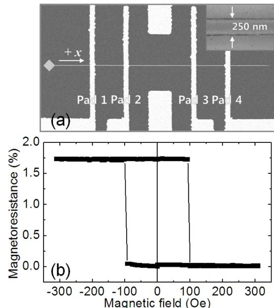
Fig. 1 (a) SEM image of spin-valve nanowire. (b) Normalized GMR curve of spin-valve nanowire
