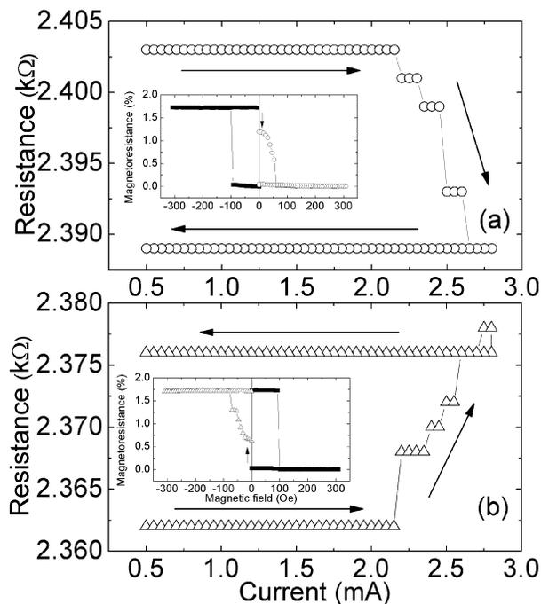
Fig. 2 Resistance at zero field in term of  $I_{\text{inject}}$  with an antiparallel (a) and a parallel configurations (b) as initial states. Insets show the GMR curve in terms of the applied magnetic field from  $H = 0$  after injection of a pulse current of 2.8 mA
