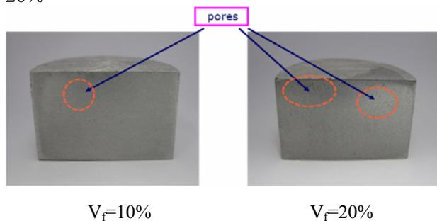
Fig. 3 The longitudinal section of MMC
