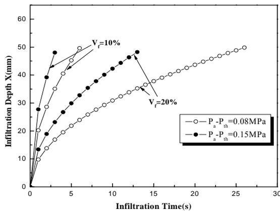
Fig. 2 Relation between infiltration depth and time.
