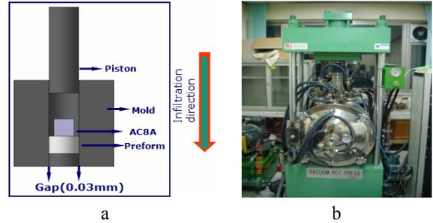
Fig. 1 (a) mold of manufacture MMC, (b) vacuum hot press
