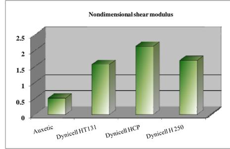
The shear strength is still considerably higher for the auxetic compared to the commercial core materials. The shear modulus was lower even though comparable. This result seems to be largely due to the use of short fibers for the specimens used in the present study.
