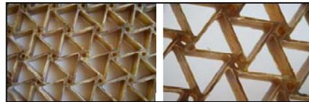
Fig.1 Examples of cellular solids with chiral geometry obtained by RTM.
