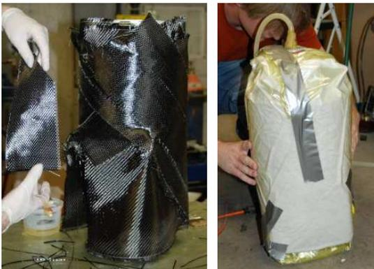
Figure 3: Wet lay-up of duct and vacuum assembly
