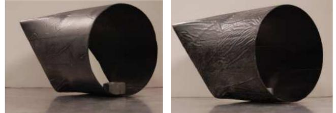
Figure 5: Finished ducts: prepreg (left) and wet lay-up
