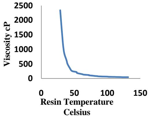
Figure 1 Pure Epoxy Viscosity
