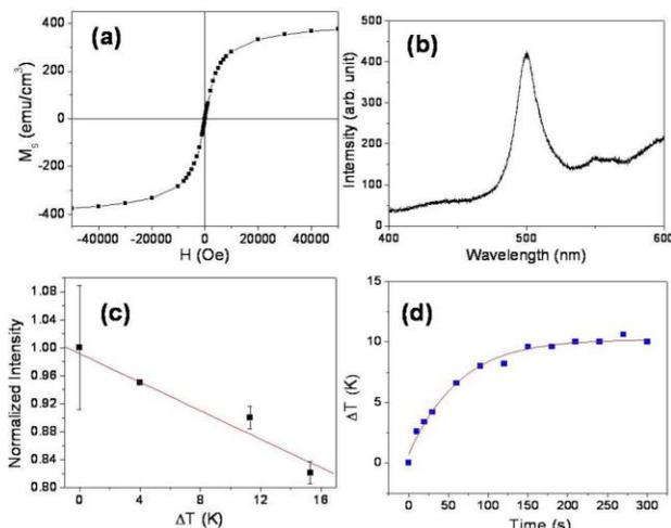
**Fig. 3** Room temperature magnetic hysteresis (a) and photoluminescence (b) of FePt/CdS heterodimer nanoparticles; integrated PL intensity as a function of temperature (c); and temperature change  $\Delta T$  as a function of time due to AC heating (d); dots are data points and the line is a guide to the eye.
