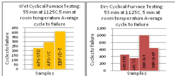
Fig 2. Wet Cyclical Furnace Test Results. Fig 3. Dry Cyclical Furnace Test Results.
