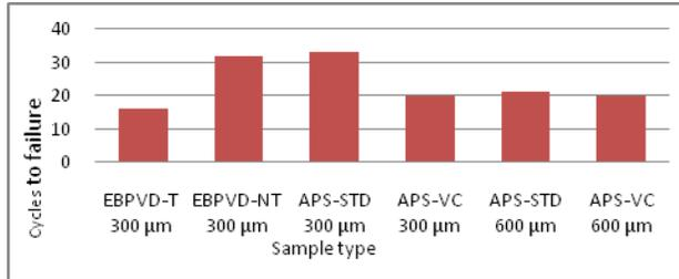
Fig.1 Thermal Cycling Spalling Resistance using 6- hour thermal cycles at 1200 ° C.
