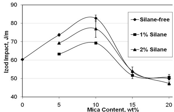
Figure 2; Effect of mica and silane addition on the Izod impact strength of the UPVC.
