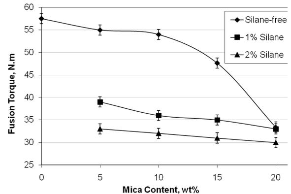
Figure 1; Effect of the mica and silane on the fusion torque of the UPVC.
