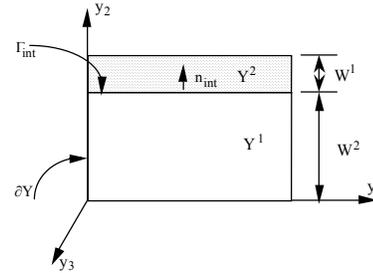
Fig. 1: Basic cell of a multilayered material with two constituents.
