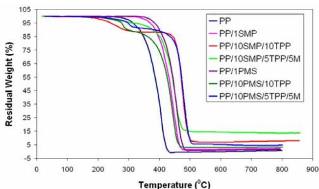
Figure 1. TGA curves of the composites in N<sub>2</sub>
