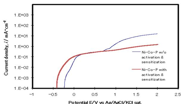
**Figure 2:** Results of anodic polarization curves for deposition in alkaline solution.
