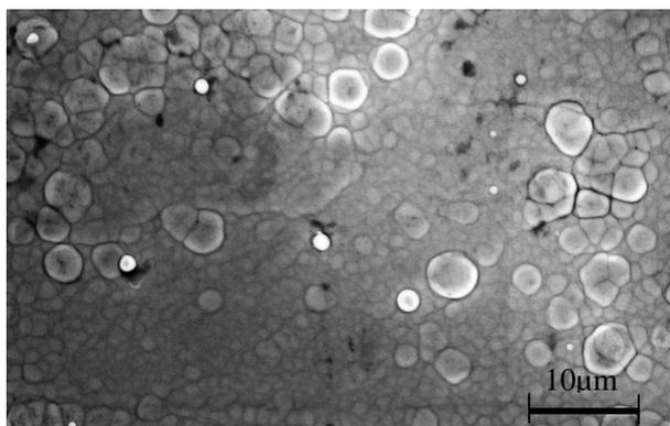
**Figure 1:** SEM micrograph of electroless Ni-Co-P coating surface without activation and sensitization.
