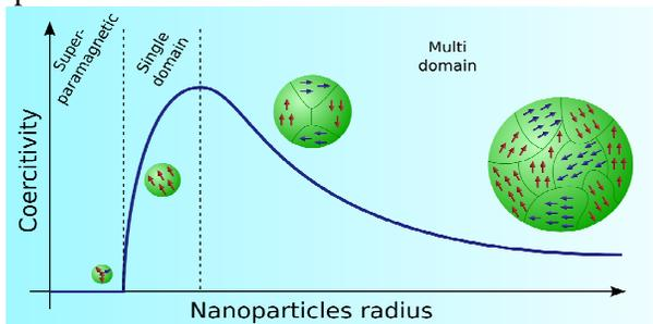
Figure 1 Schematic illustration of the coercivity-size relations of small particles.
