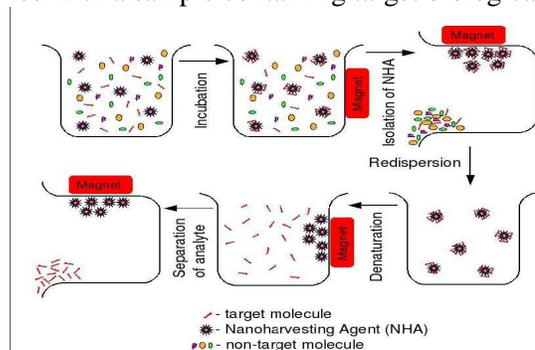
Figure 2 Separating process using functionalized “nanoharvesting” magnetic nanoparticles
