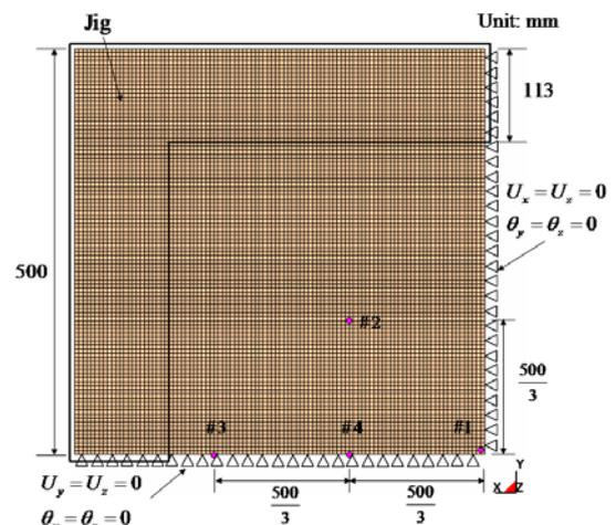
**Fig. 1** Finite element model for the multi-layered structure. The number indicates the positions for the analysis of deformation characteristics.
