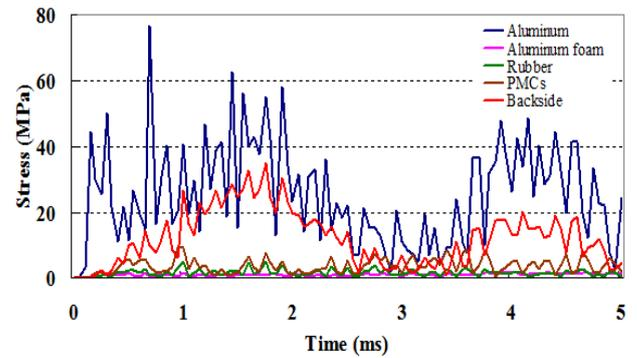
**Fig. 3** Stress variations at each layers and backside of multi-layered structure.
