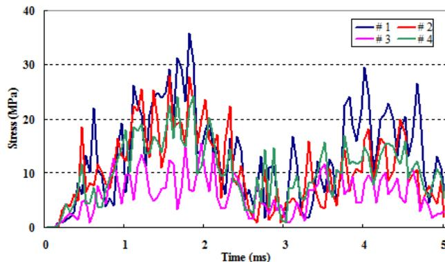
**Fig. 2** Stress variations at each position on backside of multi-layered structure.
