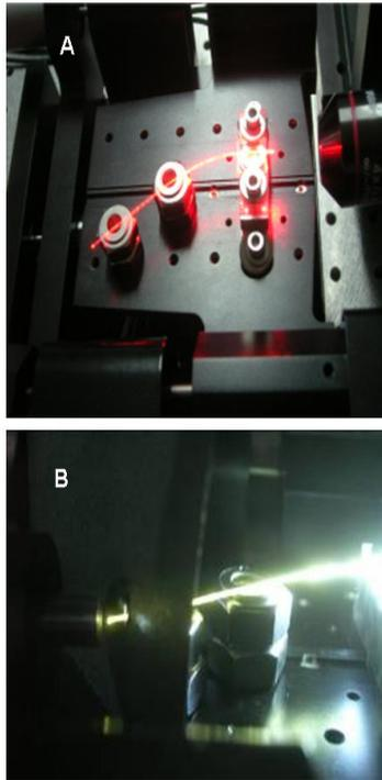
Fig. 1 Optical fiber performances of *R. racovitzae* spicules. Light transmission at 633 nm (A) and with white light generated by a Tungsten lamp (B).
