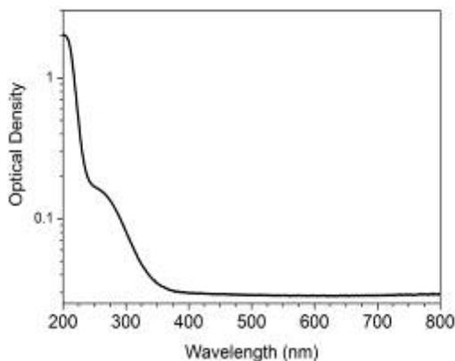
Fig. 2 Absorption spectrum of commercial silica optical materials, evidencing almost complete light-transmission in the visible range.
