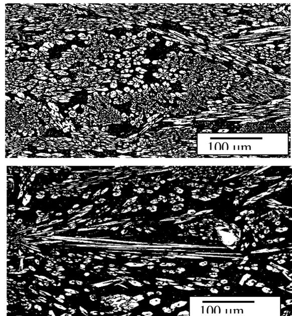
**Fig.1. Microstructure of Cobal arc hardfacing a) 4 mm and b) 6 mm thick**
