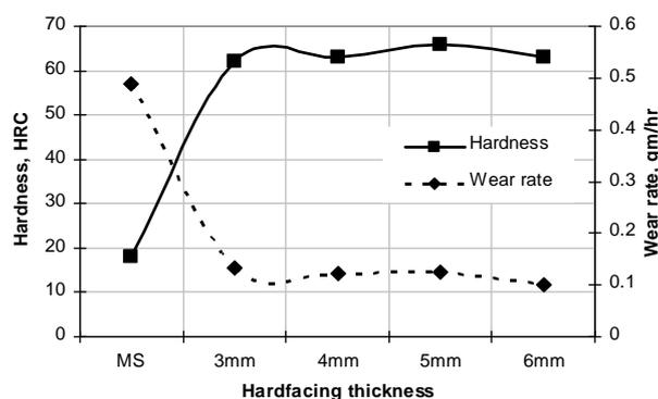
**Fig.2 Hardness and erosion rate function of hardfacing thickness**
