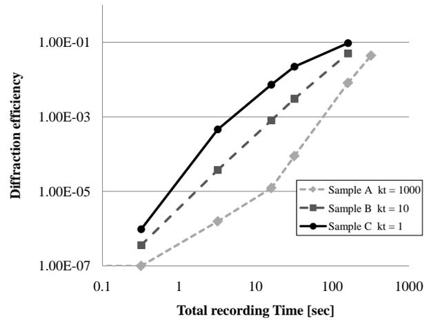
Fig.4 High-speed recording using different values of and rate constants of termination
