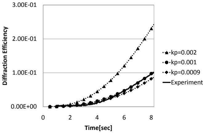
Fig. 2 Relationship between recording time and diffraction efficiency
