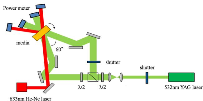
Fig. 1 Experimental setup of a two-beam interference method
