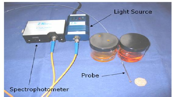
Figure 4 Experimental set up for pH monitoring probe for concrete samples
