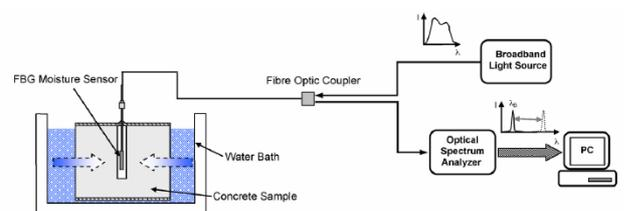
Figure 1 Moisture ingress test set up
