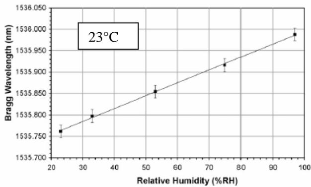
Figure 2 Calibration of the relative humidity sensor
