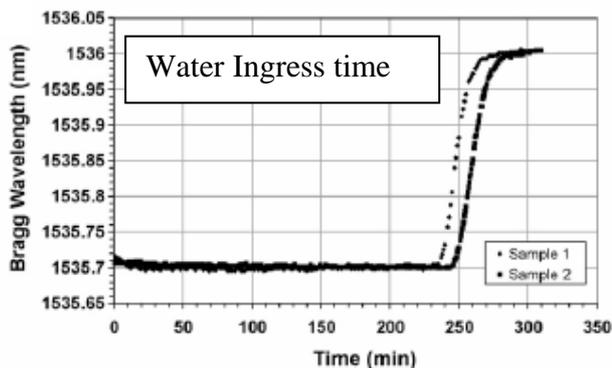
Figure 3 Water ingress time as a function of calibration wavelength (proportional to RH) for 2 samples tested
