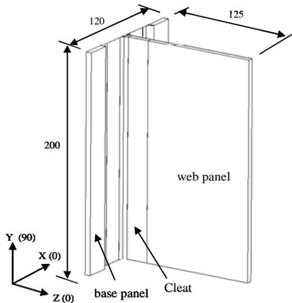
Fig. 1 T-joint structure geometrical details
