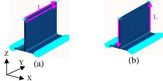
Fig. 2 FE loads and boundary conditions (a) shear load, (b) induced bending moment
