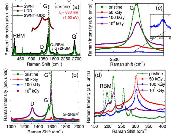
**Fig. 3.** Shown are the first- and second-order micro-Raman spectra of (a) pristine and (b, c, d) gamma irradiated nanocomposites with varying dose demonstrating the characteristic D and G band,  $G'$  band and radial breathing mode (RBM). The spectrum for UDD is also shown in (a).
