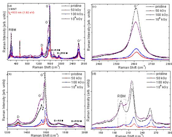
**Fig. 2.** (a) Shown are the first- and second-order micro-Raman spectra of SWCNT with varying gamma irradiation dose demonstrating the characteristic (b) D and G bands, (c) first overtone of the D band ( $G'$  band) and (d) radial breathing mode (RBM).
