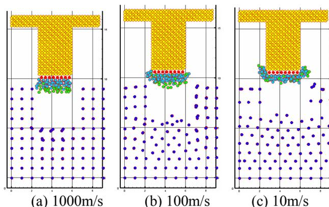
Fig. 5 Three imprint speeds for cases of 3nm width, 3nm imprint depth, and 0K.
