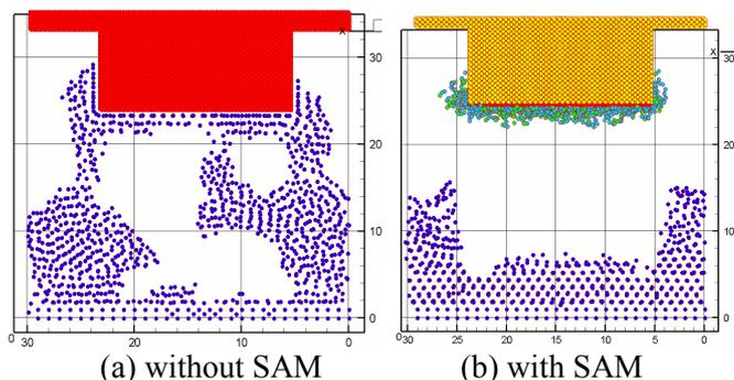
Fig. 2 Two cases of nanoimprint lithography at 300K and 1,000m/s in imprint velocity.
