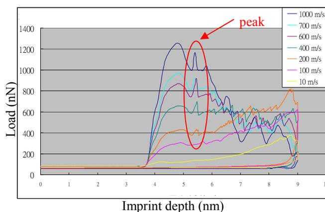
Fig. 6 Imprint speed effects on load-displacement relations for case of 3nm width, 3nm depth, and 0K.
