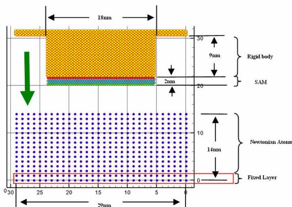
Fig. 1 Molecular dynamics model for nanoimprint lithography.
