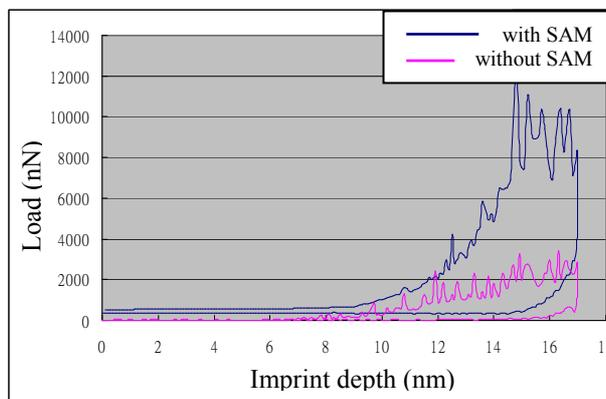
Fig. 3 Load-displacement relation with or with SAM.
