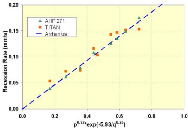
**Figure 2. Measured PICA stagnation recession rates agree with predicted values using TITAN.**
