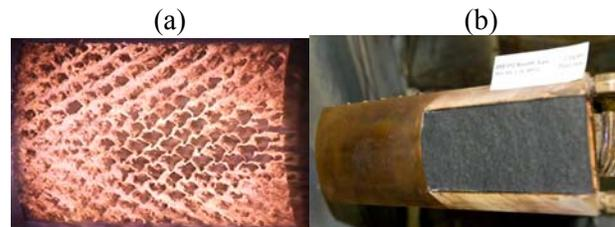
**Figure 1. (a) SLA-561V swept cylinder failure during arc jet testing, and (b) successful PICA post-test sample under same conditions.**
