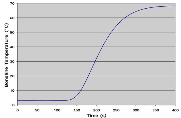
**Figure 3. Predicted bondline temperature during atmospheric entry for heatshield region with highest recession.**
