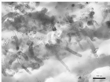
**Fig. 1** TEM picture of carbon nanotubes in SMP matrix
