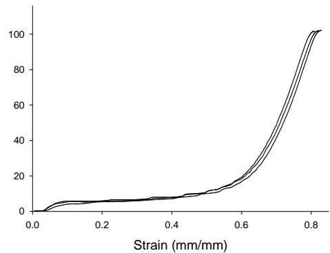
**Fig. 5** Typical compressive stress – strain curves for the foam material
