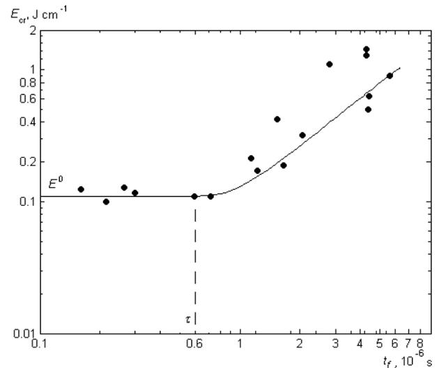
Fig. 1 Critical energy  $E_{cr}$  vs the discharge duration  $t_f$ : the incubation-time criterion (solid line) and experimental data of [5] (dots)
