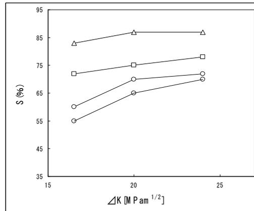
Fig.3 Ferrite selection ratio of crack path
