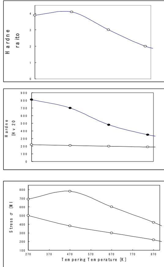
Fig.1 Relationship among hardness raito, stress and tempering temperature
