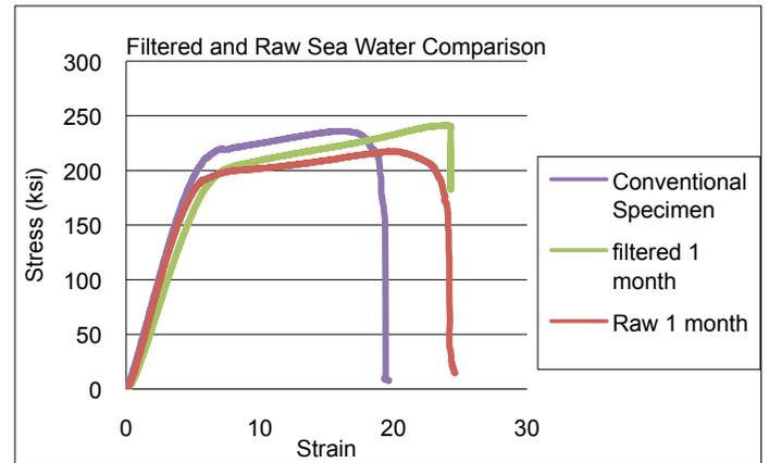
Fig. 5 Comparison of conventional, filtered, and raw sea water specimens
