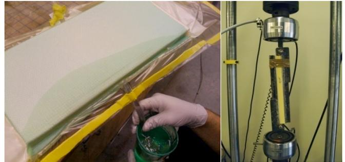
Fig.1 VRI process with resin flowing across a part
