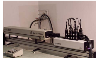
Fig. 4 Laser and Bragg Cell equipment. Fig. 5 View of LDV-PDPA laser system with for research chamber.
