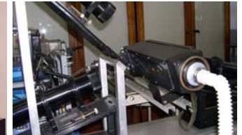
Fig. 4 Laser and Bragg Cell equipment. Fig. 5 View of LDV-PDPA laser system with for research chamber.
