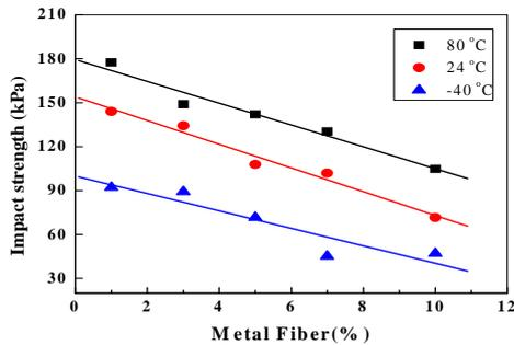
Fig. 3: Relationship between impact strength and metal fiber contents for various temperatures.
