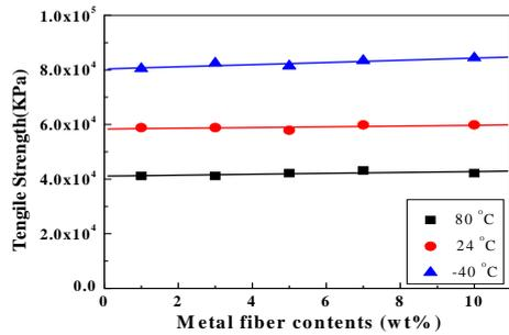
Fig. 1: Relationship between tensile strength and metal fiber contents for various temperatures.
