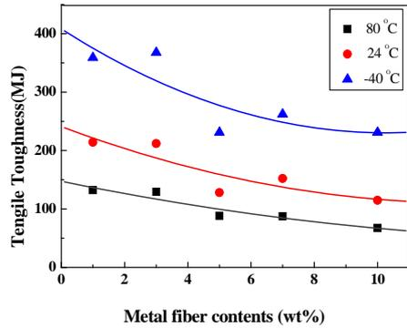
Fig. 2: Relationship between tensile toughness and metal fiber contents for various temperatures.
