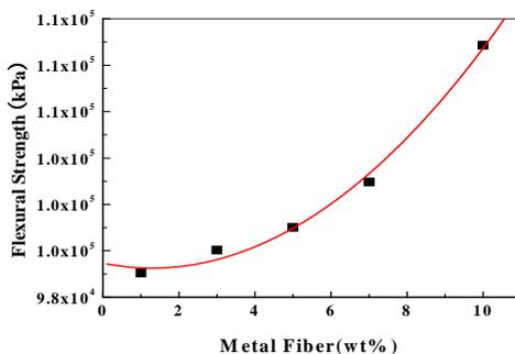
Fig. 4: Relation between flexural strength and metal fiber contents at room temperature.
