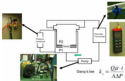
Fig.5 Transverse-plane permeability instruments
