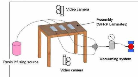
Fig. 3 In-plane permeability experimental scheme
