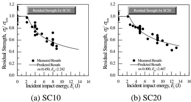
Fig. 1 Strength reduction behavior in impacted sandwich panels
