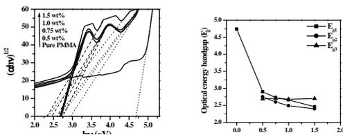
**Fig 2:** a) Plots of  $(\alpha h\nu)^{1/2}$  versus  $(h\nu)$  and b) variation of band gap with dopant concentration for  $\text{FeCl}_3$  doped PMMA films.
