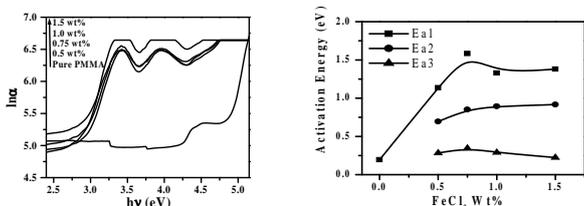
**Fig 3:** a) Plots of  $\ln(\alpha)$  versus photon energy  $(h\nu)$  and b) variation of activation energy with dopant concentration for  $\text{FeCl}_3$  doped PMMA films.
