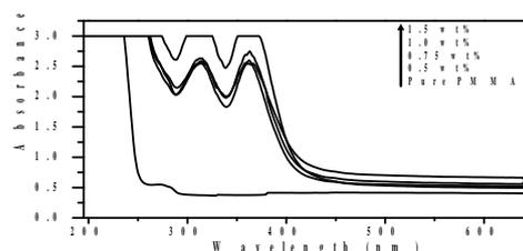
**Fig 1:** Optical absorption spectra for FeCl<sub>3</sub> doped PMMA for doping concentration.
