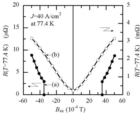
Fig. 2. Typical dependence of the resistance  $R(T=77.4\text{ K})$  on the excitation magnetic flux density  $B_{ex}$  for the sensors, under temperature conditions of 77.4 K. Here, (a) and (b) represent the characteristics of sensors constructed with (solid circles) and without (open circles) the shock compaction method, respectively.
