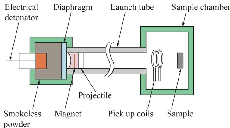
Fig.1. The shock compaction system
