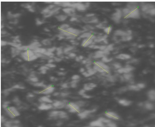
Fig. 3. The measurement of the size of crystal grain using CCD-image.
